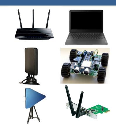
The WiFi sensing testbed includes USRP, wireless access points, laptops (with Intel 5300 and Atheros omni-directional and directional AR9580),
