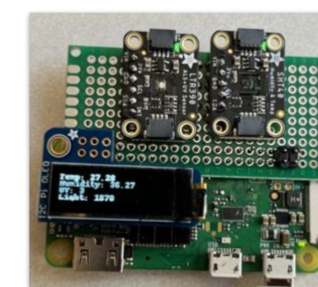
Raspberry Pi based climate sensor
