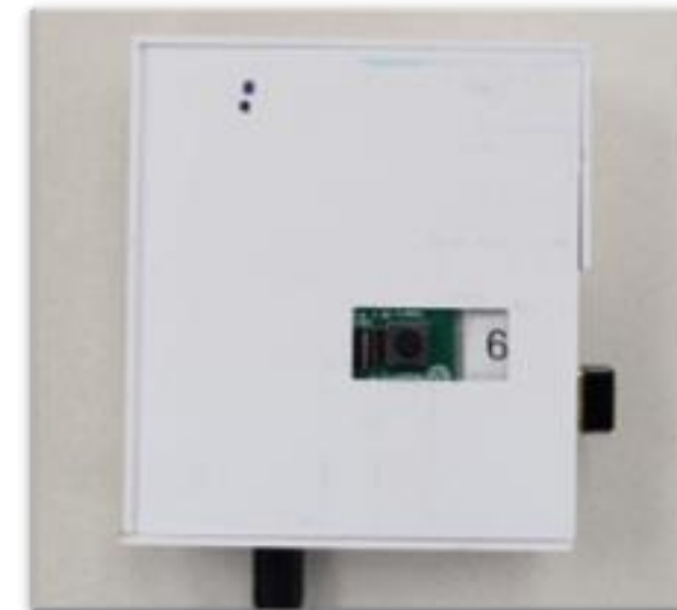
Self-built Raspberry Pi based video doorbell
