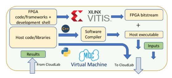
2. Deployment: After creating the bitstreams/host executables, users will use CloudLab for targeting. There are eight Alveo U280s in CloudLab Massachusetts cluster which are PCle connected to eight host machines. The U280s are connected to a 100 GbE data center switch using 100G QSFP28 passive DAC cables.
